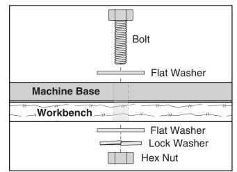
Figure 9. Example of a through mount setup.
